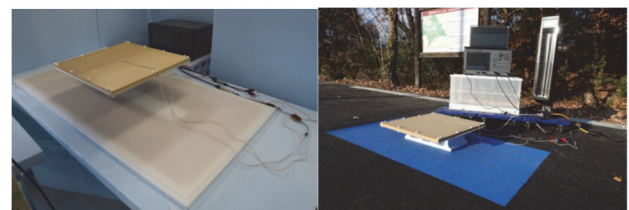
Fig.2 Transmitting and receiving coils' measurement environments before and after burial
